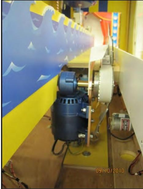
The profile ducks are fastened to a toothed timing belt, driven by a geared motor which runs continuously when the machine is connected to a power supply. Four electrical solenoids are spaced at equal intervals in front of the ducks, and trip the ducks over when the target is hit and the tripping mechanism is in line with a duck.
